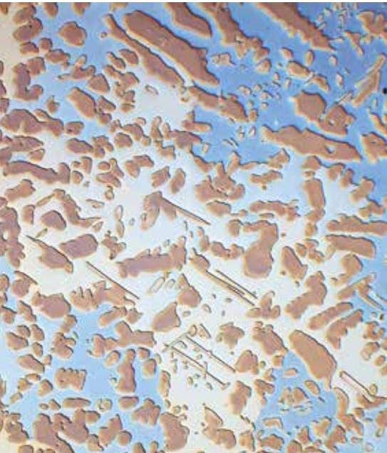
Duplex stainless steel, etched electrolytically using 40% aqueous sodium hydroxide solution. Differential Interference Contrast, 100x.
