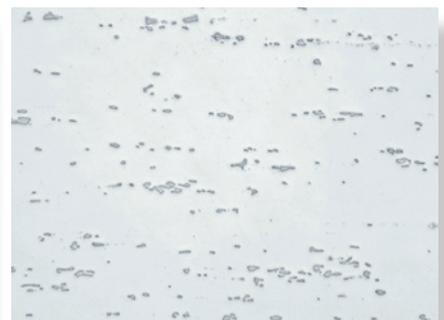
Fig. 5: As Fig. 4, hot rolled, unetched, 200x.
