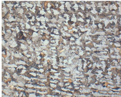
Fig. 7: C45 steel etched with 3 % Nital. The white phase is ferrite and the rest is pearlite. Optical microscope. Bright Field (BF), original magnification 200x.
