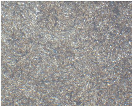
Fig. 17: Martensite in a tool steel (9CrWMn) etched with 3% Nital. Optical microscope. BF, original magnification 500x.
