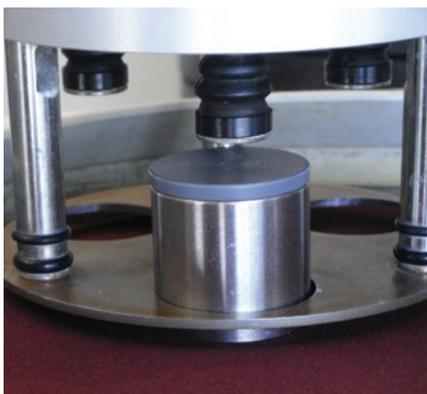
Fig. 5: Holder with specimen ready for polishing.
