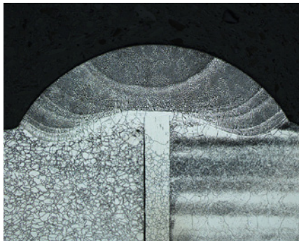
Mechanically polished and electrolytically etched section through micropulse Tungsten Inert Gas weld in Inconel 625 alloy. Etched in 10% oxalic acid; 10 Volts for 10 secs. Bright field, 2.5x.
