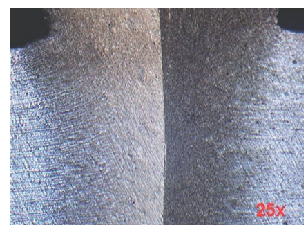
Fig. 3: Fusion interface on pressure friction welded low alloy steel showing heat affected zone and associated plastic deformation. Bright field, 25x.
