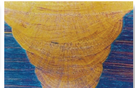
Polished and colour etched section through a multi pass austenitic stainless steel weld. Colour etched according to Lichtenberger and Bloech. Bright field, 6.5x.
