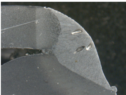
Sub surface gas porosity in automatically MAG (Metal Active Gas) welded steel components. Ground and etched with 10% Nital. Bright field, 2x.
