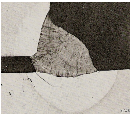
Heat affected zone crack below fillet weld in low alloy steel. Bright field, 5x.
