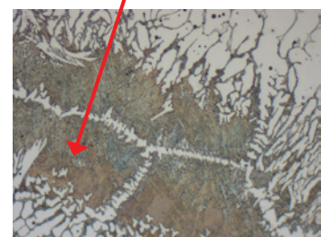
Polished and etched section of austenitic stainless steel weld showing islands of delta ferrite and small area of pearlite.
