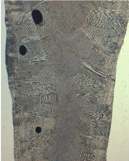
Cross section through electron beam weld in nickel base alloy showing a welded columnar microstructure with few scattered gas pores. Bright field, 50x.
