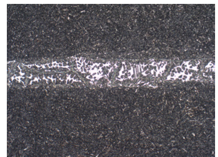
Fig. 6: Tempered martensitic stainless steel with delta ferrite, etched with picric acid 75x
