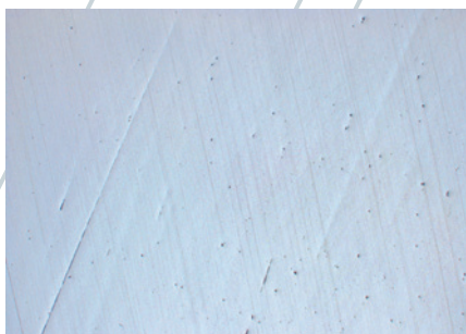
Surface of stainless steel after 3µm polish, showing deformation from grinding DIC 25x
