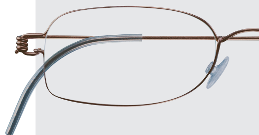
Details of a titanium frame for eye-glasses. The high strength and ductility of titanium make screws and solder on these frames obsolete.
