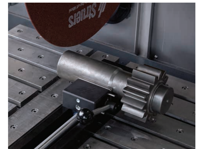
Base plate tool right 12 mm with prism jaws.
