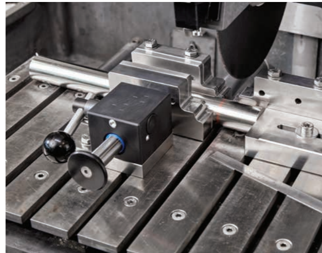
Quick clamping tool with prism jaws and adjustable stop for serial cutting.
