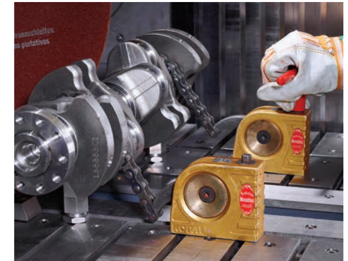
Vertical clamping tools with chain spanners.
