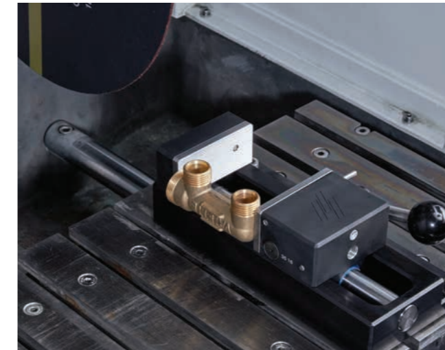
Base plate clamping tool with grooved jaws.
