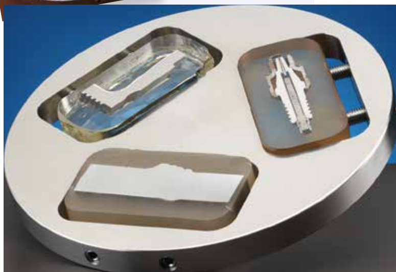
The specimen holder with rectangular holes can hold specimens up to 70x53 mm
