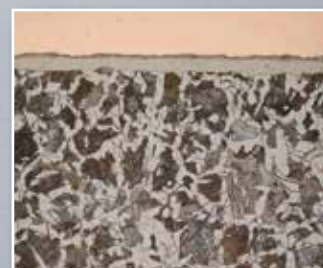
Coating - measure thickness of coatings on metals, according to standard.
