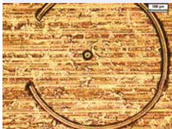
Chromium PVD layer on steel, possible corrosion site, 50 x
