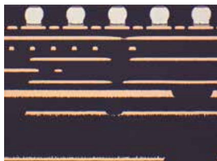
BGA solder ball, cross section, 100x
