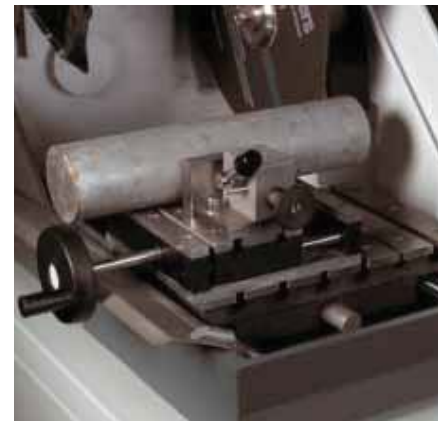
Adjustable cutting table for cutting many similar specimens (optional)
