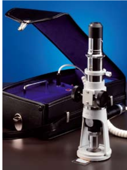
PSM-2 and Transcopy constitute an indispensable tool for non-destructive materialography.
