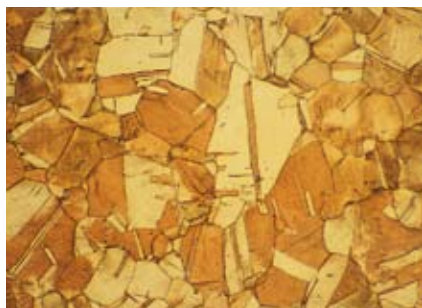
Pure copper. Sample etched with cupric chloride and ammonia. Magnification 100 x
