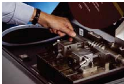
Built-in convenience: Flush hose for cleaning of the cutting chamber
