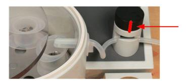
The groove (line) on the valve must face the front of the machine.
