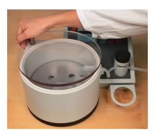
Ensure that the lid is directly over the chamber and that there are no leaks around the edges. Should some leaking occur, release the vacuum, reposition the lid and reapply vacuum.
