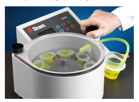
■ When all cups have been filled, press stop to release the vacuum.
