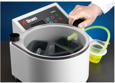
■ When the specimen is covered with impregnation material, turn off the flow, turn the holder so that the next mounting cup is under the dispensing tap and repeat the filling procedure. Repeat until all mounting cups have been filled up. If necessary, refill the mixing cup with impregnation material.
