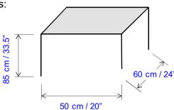
To take advantage of the maximum spindle capacity, a hole must be drilled in the table top to accommodate the full stroke of the spindle. Please refer to the *Drilling Plan* for dimensions.
