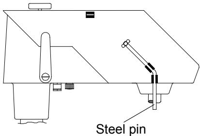
To avoid directional abrasion of the specimens during preparation LaboForce-Mi is equipped with the ability to carry out forced rotation of the specimens.
