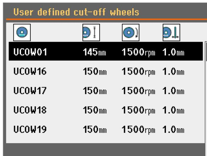
The screenshot shows a table of user-defined cut-off wheels. The table has four columns: ID, Diameter, RPM, and Thickness. The first row is highlighted.
