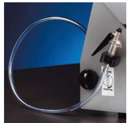
The flush hose facilitates cleaning
