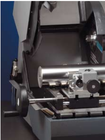
The adjustable cutting table enables parallel sectioning
