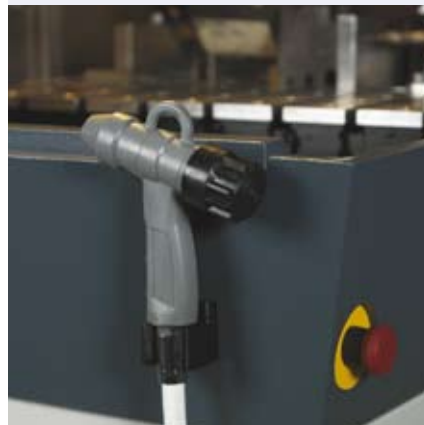
Flushing gun for cleaning the cutting chamber.
