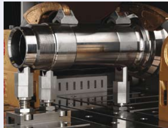
Adjustable support blocks (turnable, horizontally and vertically adjustable), and vertical clamping tools (optional Arm Extension).
