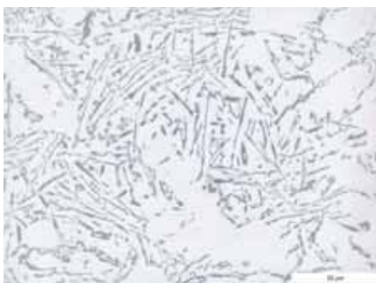
Fig. 7: Aluminium-silicon cast, unrefined, 500x.
