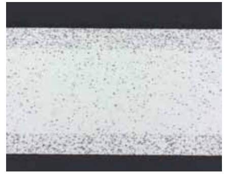
Plated sheet, core: aluminium alloy 3503, plating: aluminium alloy 4104, unetched 100x.
