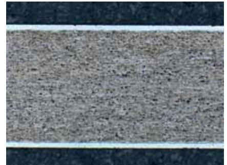
Plated sheet, core: aluminium alloy 2024, plating: aluminium 99.5%, etched with Dix and Keller, 50x.
