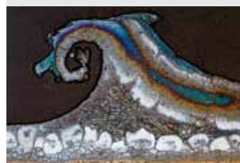
Fig. 17: Burr on a solder spot of a heat exchanger, pre-etched with sodium hydroxide, colour etched with potassium permanganate according to Weck.
