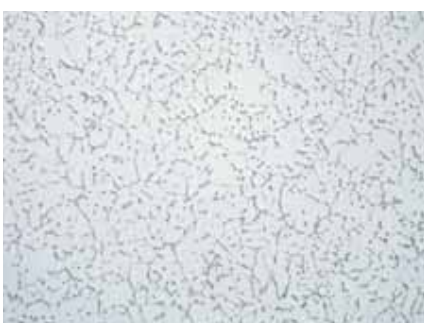
Fig. 3: Aluminium alloy 2024, cast, showing eutectic precipitation on grain boundaries, unetched, 200x.
