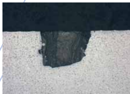
Fig. 2: Oxide in the surface of an aluminium pressure die casting, 50x.
