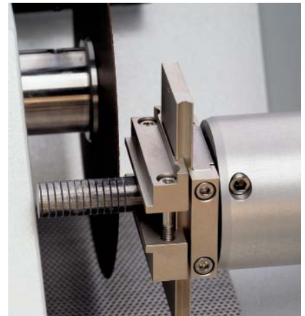
Accutom-50 can be programmed to automatically cut series of slices from the same samples
