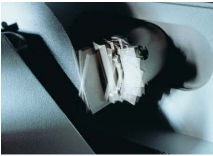
Oscillating movement is used for cutting oblong samples, thus reducing the cutting time considerably
