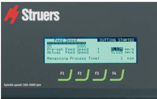
After the process has been started, the display changes and the relevant parameters are shown
