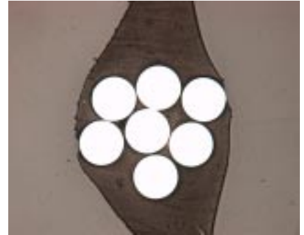
Cord 1a. Same picture as MD-Chem, but Bright field illumination, notice that the visibility of the rubber penetration is not as good as in the Dark Field image.
