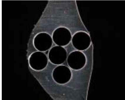
MD-Chem. Dark Field illumination, sample after final polishing stage
