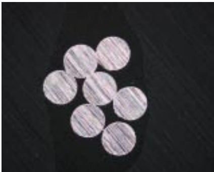
Grinding. Dark Field illumination, sample after grinding
