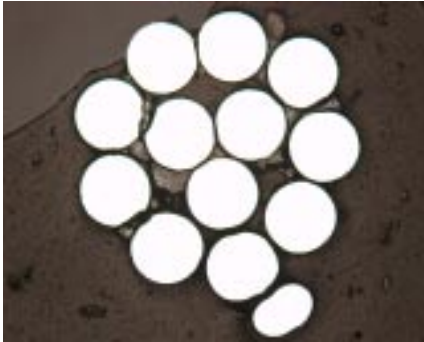
Cord with fretting. Bright field illumination. Damage on cord filaments, fretting corrosion products in cable.
