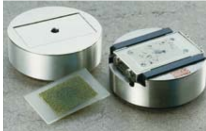
Thin section holders for lapping and polishing
