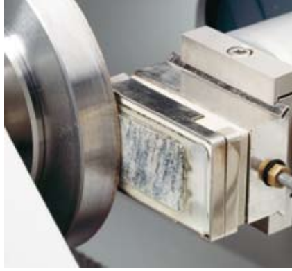
Grinding with cup-wheel on Accutom-50
