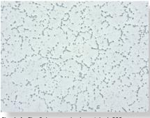
Fig. 4: As Fig. 3, homogenised, unetched, 200x.
