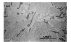
Fig.15: Experimental aluminium alloy with 6% Si and 10% copper, unetched
