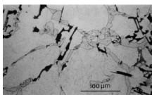
Fig. 16: Same as Fig. 15 but etched for 30 sec with 1g molybdic acid in 200 ml water + 6 g ammonium chloride. The silicon is dark blue and is distinguishable from the arevish CuAl
