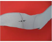
Fig. 13: Pressed part, macro etching, primary and heterogeneous precipitates are revealed that have a negative effect on the surface of the final product.
