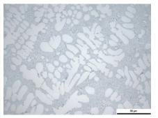
Fig. 8: Aluminium-silicon cast, refined, 500x.
