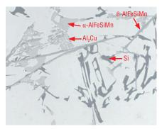
*Fig. 6: AlSi6Cu4 cast, the various phases can be identified by there typical colour.*
