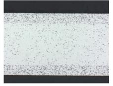
Plated sheet, core: aluminium alloy 3503, plating: aluminium alloy 4104, unetched 100x.
