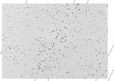
Fig.1: Embedded diamond particles in pure aluminium after polishing with 3 μm, 200x.
