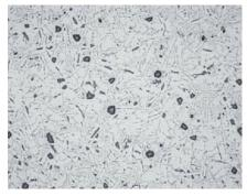
Fig. 11: Aluminium-silicon cast polished too long with OP-S suspension, silicon precipitates stand in relief, 100x.
