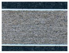
Plated sheet, core: aluminium alloy 2024, plating: aluminium 99.5%, etched with Dix and Keller, 50x.
