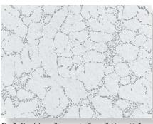
Fig. 9: Aluminium-silicon cast, after polishing with 3µm diamond small scratches are still visible, 200x.
