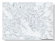
Fig. 7: Aluminium-silicon cast, unrefined, 500x
