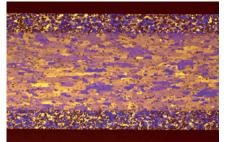
Fig. 12: Plated sheet, anodised, grain areas are clearly visible and suited for automatic image analysis, polarised light with  $\lambda$ . $\mathcal{V}$ -plate, 100x.
