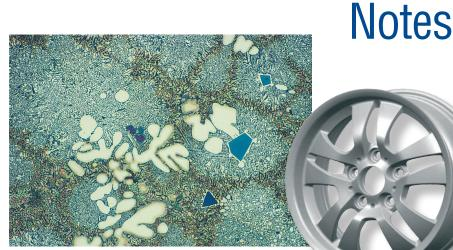
Aluminium-silicon cast, colour etched with molybdic acid, 200x.
