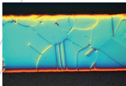
Fig. 2: Same sample as Fig.1 with final polish of OP-S-ammonia water-hydrogen peroxide-mixture, DIC, 200x.
