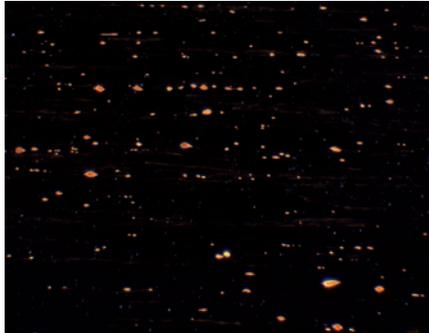
Fig. 5: Copper with red copper oxides,
