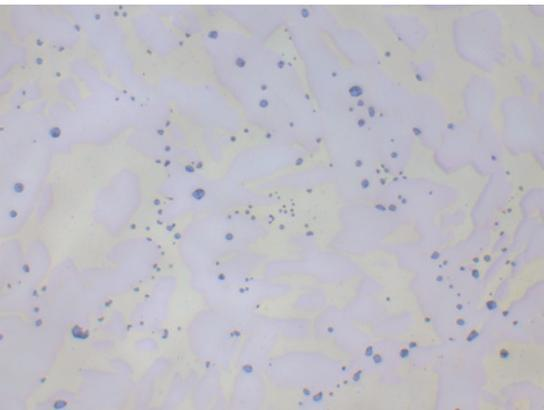
Fig. 11:  $\alpha$ - $\beta$ -brass cast (CuZn40Pb2) with grey-blue lead inclusions, unetched, 500x.
