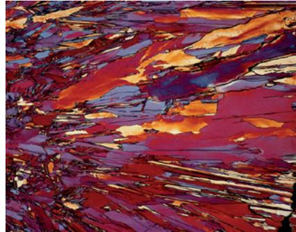
Fig. 7: Copper cathode, etched according
