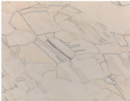
Fig. 6: Oxygen free copper, etched with ammonium
