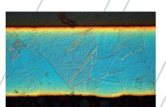
Fig.1: Pure copper wire, with final polish of OP-S, DIC, 200x.
