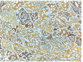
Fig.12:  $\alpha$ - $\beta$ -brass cast, etched according to Klemm, light  $\alpha$ -solid solution in dark matrix of  $\beta$ -solid solution, 100x.
