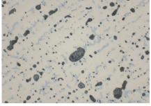
Fig.17: Bronze cast, CuSn8Pb, unetched, large and small blue-grey lead inclusions, pale blue α-δ eutectoid discernable. 500x.
