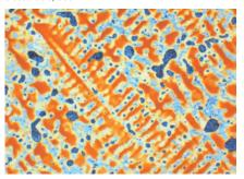
Fig.18: Same specimen as in Fig.17, colour etched according to Klemm, dendritic structure with light blue eutectoid and blue lead inclusions. Small lead inclusions can not be clearly differentiated, 500x.
