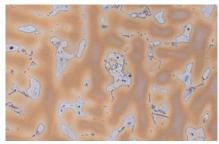
Bronze cast, CuSn10, etched with iron (III) chloride, dendritic structure  $\alpha$ - $\delta$  eutectoid, 200x.
