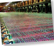
Fig. 3: Electrolytic refining
