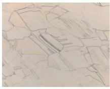
*Fig. 6: Oxygen free copper, etched with ammonium peroxydisulfat, 100x.*
