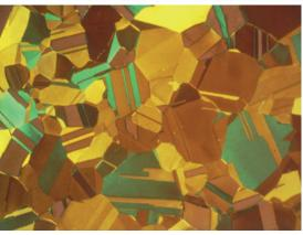
Fig. 10: α-brass, colour etched, 200x.
