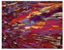
Fig. 7: Copper cathode, etched according to Klemm, 100x.
