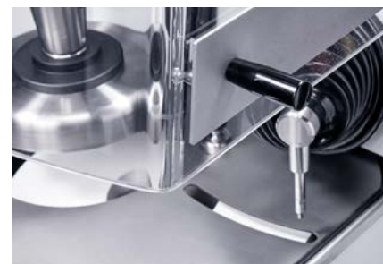
On AbraPlan-30, grinding stones of 356 mm dia. are used. This allows for the preparation of specimen holders up to 200 mm dia., which again makes it possible to prepare large or many specimens in a very short time.
