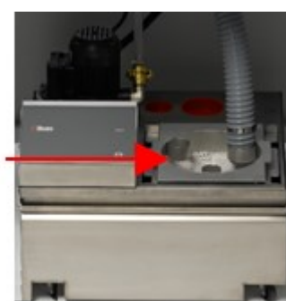
A Static filter unit
