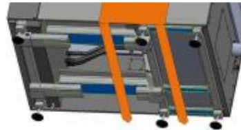
Lift from front (recommended)
