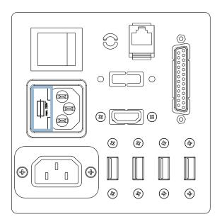
The fuse holder is located directly over the power socket at the rear of the machine.
