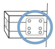
• Unscrew the six screws securing the transport safety plate at the rear. Use a 2.5 mm (0.1") Allen key.
