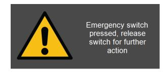
The machine stops and a message is shown prompting you to release the emergency stop. If this does not happen, contact Struers Service.
