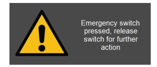
If the emergency stop is activated during start-up, an error message is shown.
