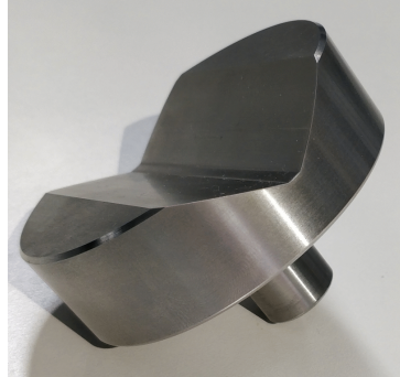
V-type anvil for cylindrical samples (option).
