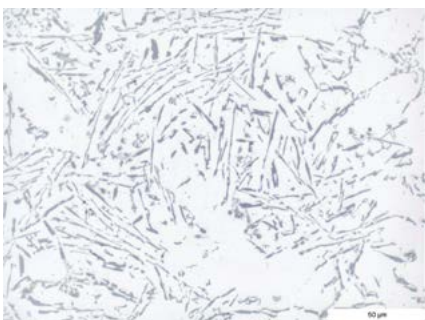
Fig. 7: Aluminium-silicon cast, unrefined, 500x.
