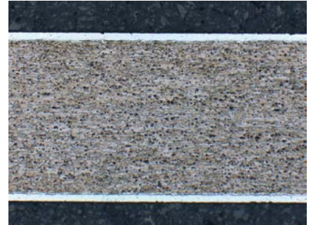
Plated sheet, core: aluminium alloy 2024, plating: aluminium 99.5%, etched with Dix and Keller, 50x.
