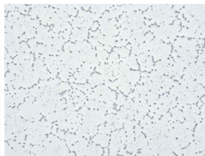
Fig. 4: As Fig. 3, homogenised, unetched, 200x.
