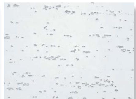
Fig. 5: As Fig. 4, hot rolled, unetched, 200x.
