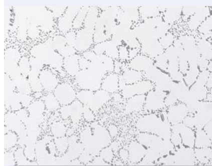
Fig. 10: Structure as in Fig. 9, but fine polished with OP-U suspension. The matrix is well polished and the eutectic has more contrast, 200x.
