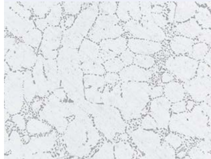
Fig. 9: Aluminium-silicon cast, after polishing with 3µm diamond small scratches are still visible, 200x.
