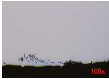
Fig. 3: Grey oxide (defect) rolled into surface of bar.
