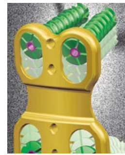
Fig. 5: Screws and bone plate electro-chemically oxidized for colour coding. The colours are the result of different thickness of the oxide layer.
