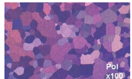
Fig. 8: Cross-section of bar, commercially pure titanium, electrolytically polished, 100 x, polarized light.
