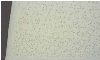
Fig. 7: Titanium after 3 μm diamond polish, deformation and scratches are not removed.
