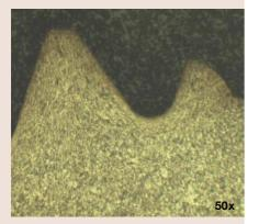
Thread of bolt, alloyed steel tempered Etchant: 3% Nital
