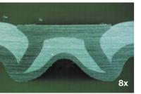
joint, steel rivet in aluminum
