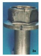
Fig. 7a: Split in head of carbon steel bolt caused by a seam.
