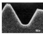
Section of thread showing decarburization Etchant: 5% Nital
