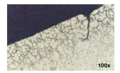
Fig. 8: Melted grain boundaries due to overheating in heading. Nickel base alloy Etchant: modified Kalling's
