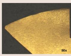
Head of brass screw with flow lines from cold forming. Etchant: Iron (III) chloride
