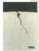
Fig. 7b: Traverse section of the seam in the fig. 7a. Echant: 3% Nital
