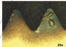
Thread, staining due to shrinkage gap
