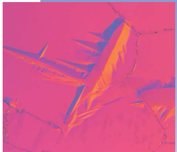
Plastic mould steel etched with 5% Picral, revealing some singular needles and plates at high magnification in an otherwise amorphous martensite
