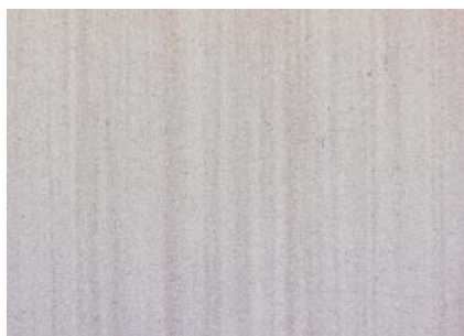
Fig. 8: Hot work tool steel showing segregations 100x
