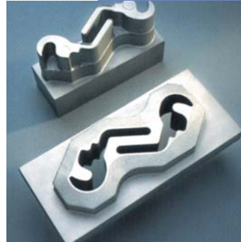
Cold work tool steel. Tool for punching
