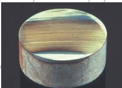
Fig. 1: Thermal damage due to faulty cutting conditions
