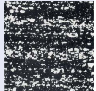
Fig. 11: Carbide distribution in conventionally produced steel
