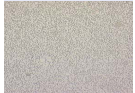
Fig. 10: Plastic mould steel after annealing shows very fine carbides 500x
