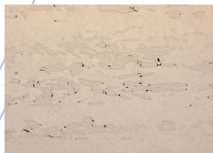
Fig. 2: Fractured primary carbides
