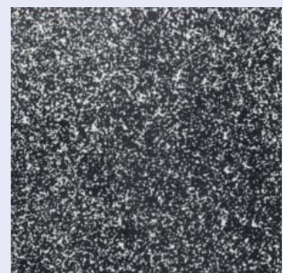
Fig. 12: Carbide distribution in powder metallurgically produced steel
