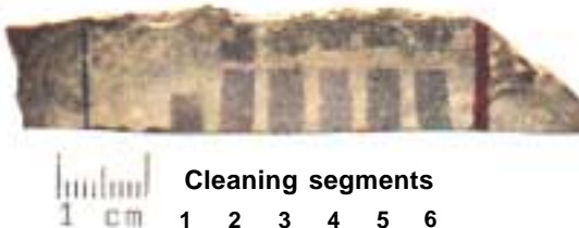
Fig. 5. Glass sample from Window n III, Cologne Cathedral showing the test cleaning zones
