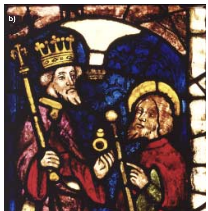
Fig. 12a/b. Photograph taken with transmitted light of a segment of medieval stained glass from Erfurt Cathedral (1405) before (a: left) and after removal of the corrosion-induced crust with cleaning compresses (b: right)
